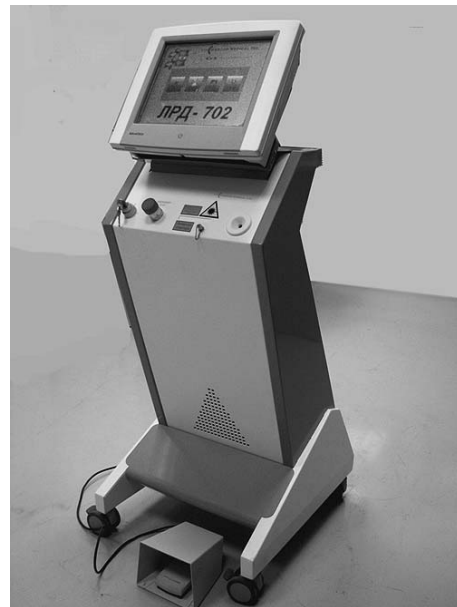
Fig. 10. Photograph of the LRD-702 laser reconstructor of the discs.
